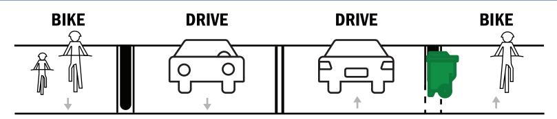
Mountable curb will be installed to facilitate heavy trash pickup at standard roadway edge location.
